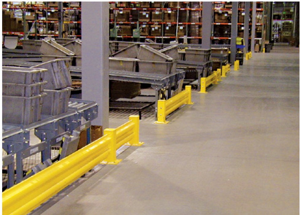
Photo: Equipment Protection Single Rail Guardrail
