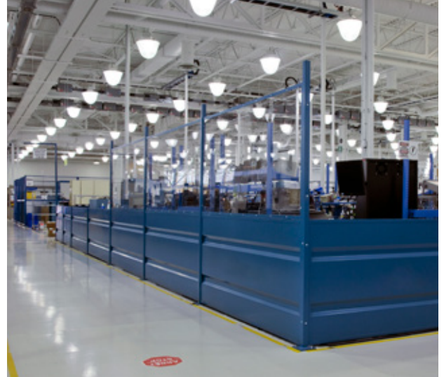
Photo: Sheet Metal & Lexan Workspace Division Partition
