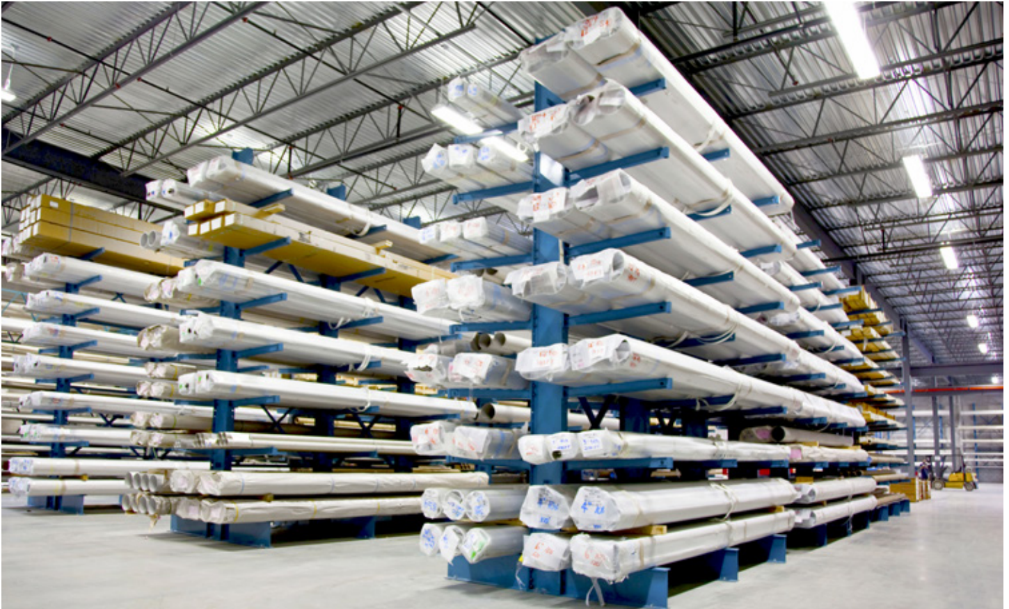
Photo: Cantilever Racking for Metal Tube & Piping Storage
