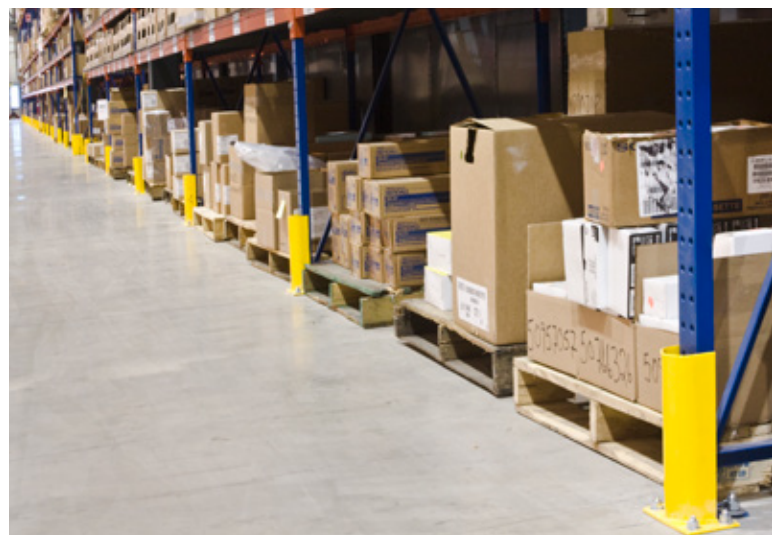
Photo: Rack Post Protection Guards
