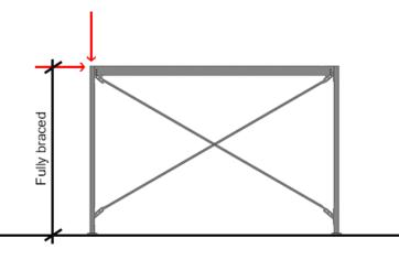
An x-brace design is virtually the least expensive brace design for medium to big sized mezzanines. Since
