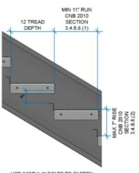
USE 3/8"Ø X 1" BOLTS TO FASTEN STEPS ONTO THE STRINGERS USING PRE-PUNCHED HOLES
