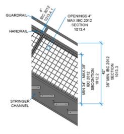
ALL GUARDRAILS, GURADRAIL UPRIGHTS AND HANDRAIL ARE HSS 1 1/2" X 1 1/2" X 16GA. THE ENTIRE SYSTEM [i.e. ALL GURADRAILS, GUARDRAIL UPRIGHTS AND HANDRAILS] ARE SHOP WELDED YO THE CHANNEL STRINGER
