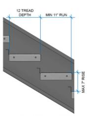
USE 3/8"Ø X 1" BOLTS TO FASTEN STEPS ONTO THE STRINGERS USING PRE-PUNCHED HOLES
