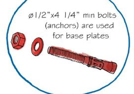
Drive the hilti bolt in the hole so that at least 6 threads are below the top surface of fixture.
