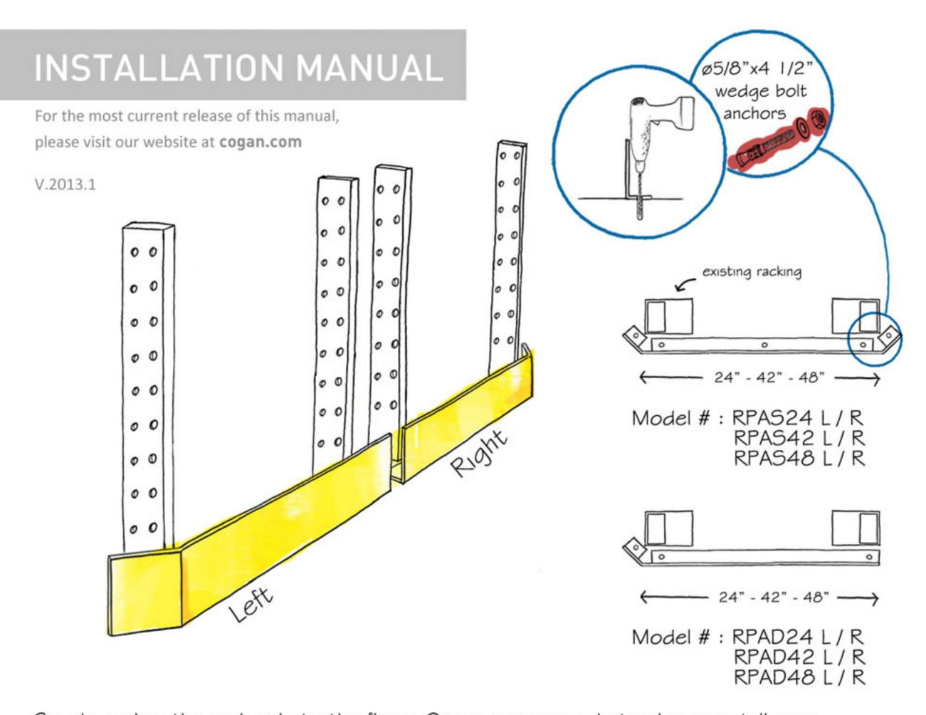
Simply anchor the rack pals to the floor. Cogan recommends to always install on a concrete surface.
