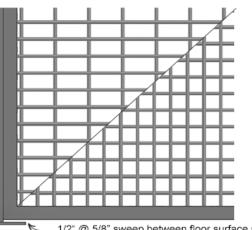
ALL DEA cage panels are mounted flush to the floor (1/2" sweep) on 2" x 2" posts.
