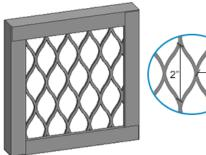
Flattened expanded metal 10GA with 1" x 2" diamond shaped openings
