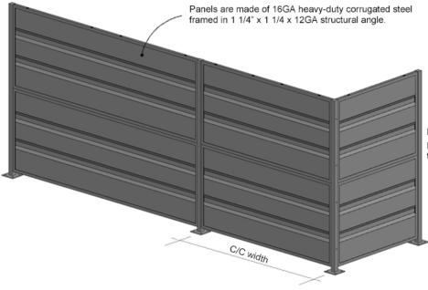
Panel dimensions are based on center-to-center post spacing. To calculate exact panel width apply the following:
